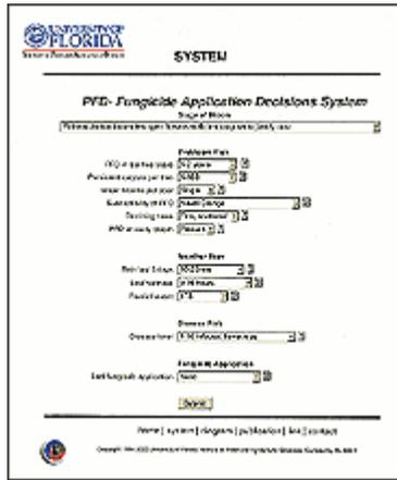
Fig. 3. The PFD-FAD input screen. Users make selections from pull-down lists and then submit to obtain a recommendation.
