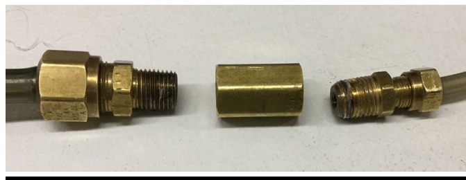
FIGURE 4 Brass airline compression fittings and coupler used to connect backpack hose to syringe hose.
